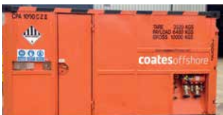
Successful testing with Petrofac: 1000cfm Containerised Zone II Air Compressor
